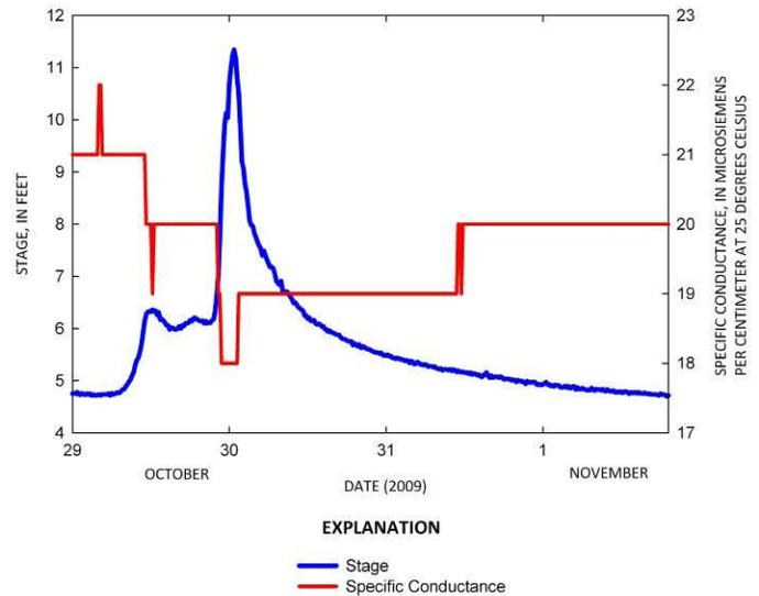
**Figure 8.** Comparison of stage and specific conductance for 07075250.
