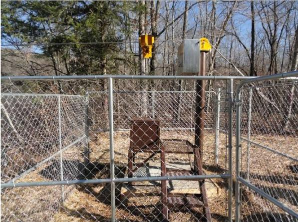
**Figure 6.** Bank operated cableway installed at the gaging station 07075250.
