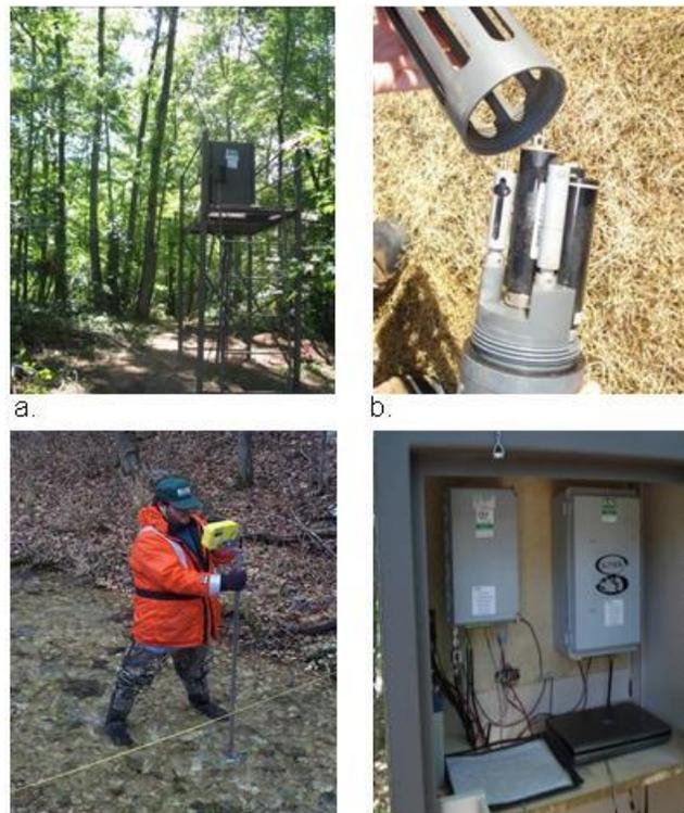
**Figure 5.** a. Continuous water quality monitor and streamflow gaging station site 07075250 gage shelter; b. Continuous water quality monitor; c. USGS hydrologist conducting streamflow measurement; d. Data collection instrumentation inside gaging station.
