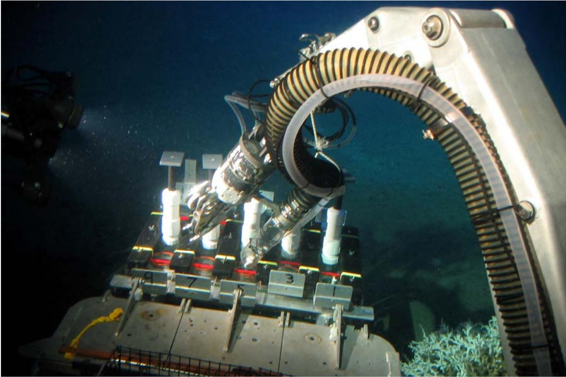
Figure 6.4. The ‘Kellogg Sampler’. This specially designed microbial isolation/sterility box with multiple chambers is used to collect discrete *Lophelia* samples for coral microbial ecology experiments.
