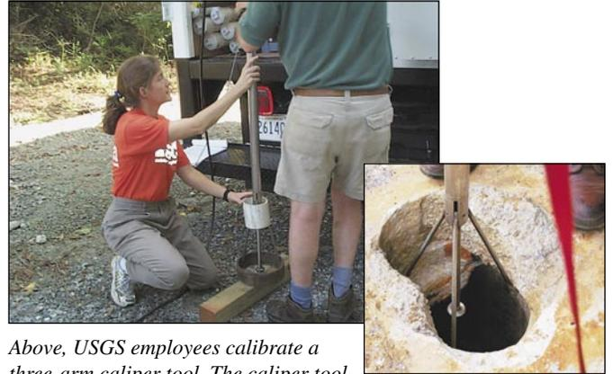
Above, USGS employees calibrate a three-arm caliper tool. The caliper tool (right) measures diameter by pressing mechanical arms out against the borehole wall. Geophysical tools measure the physical properties of the rock surrounding the well. Photo by Lester J. Williams, USGS.
