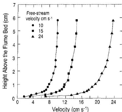
**Fig. 2.** Profiles of streamwise velocity above flume bed. Velocity profiles made at upstream edge of test section show presence of well-formed boundary layers and, depending on free-stream velocity, markedly different flow rates in layer <0.5 cm above bed, i.e., layer from which the clams feed
