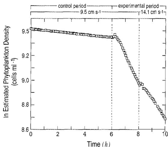
**Fig. 3.** *Chroomonas salina*. Variation in estimated phytoplankton abundance with time. Rate of decrease in cell density increased dramatically when clams (*Potamocorbula amurensis*) were added to system at Hour 6 and then slowed when flow velocity was increased to  $14.1 \text{ cm s}^{-1}$  at Hour 8. Each data point represents average cell density for a 5 min interval, based on continuous measurement of in-vivo fluorescence
