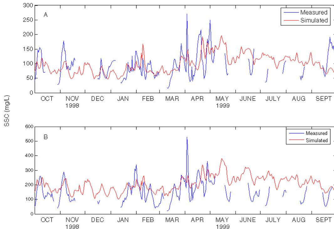
Figure 3 Simulated SSC for water year 1999 at Dumbarton Bridge (A) at mid depth (22 ft below MLLW) and (B) at near bottom (41 ft below MLLW).
