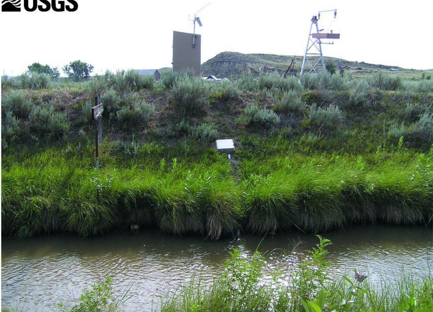
Prairie Dog Creek near Acme, Wyoming, July 2004. The gage house (middle) and cableway (right) are on the higher terrace in the background. The cantilever gage (left) and box (middle) to access the continuous specific-conductance monitor are on the lower terrace in the foreground.
