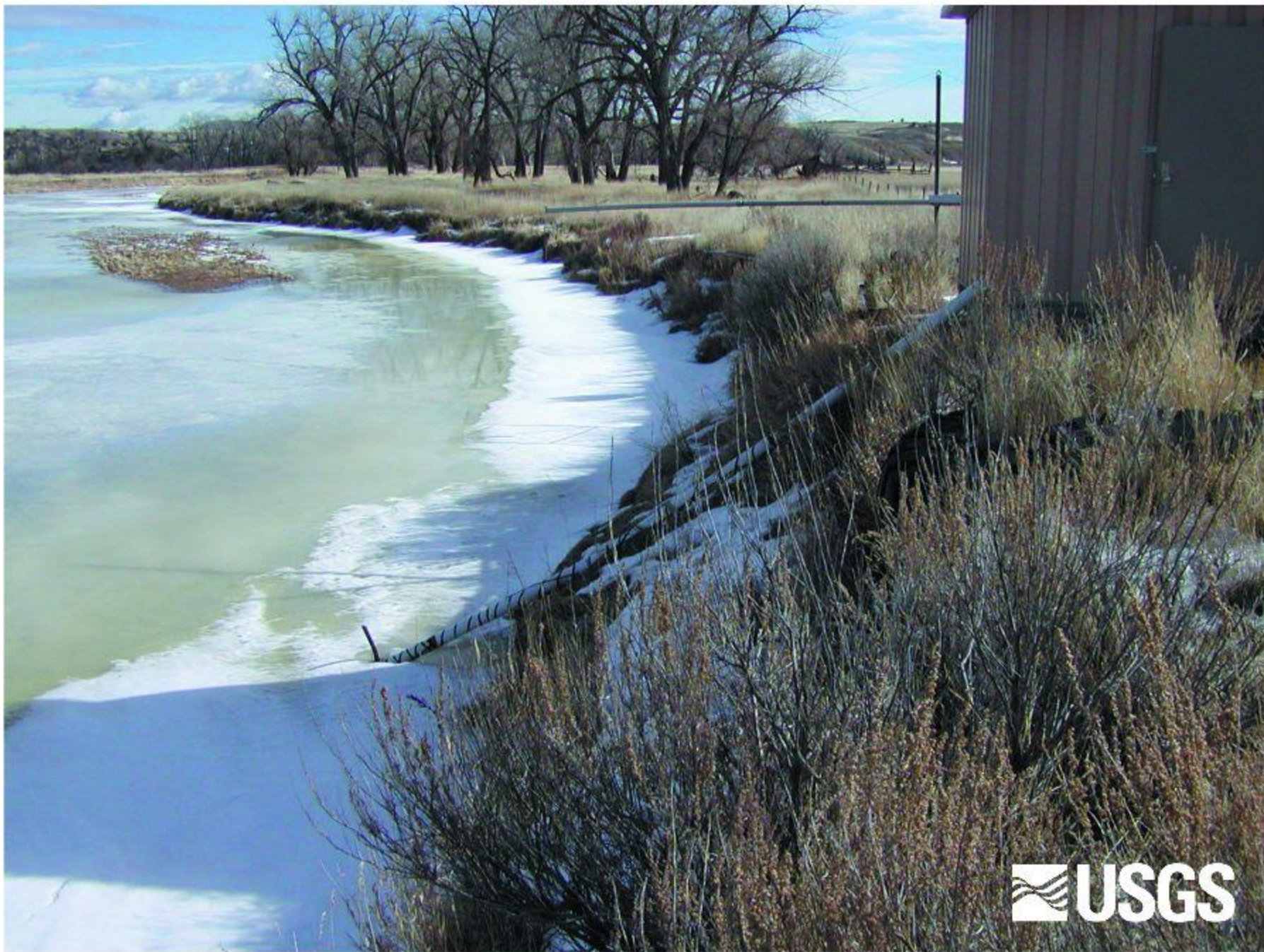
Tongue River at State Line, Montana, February 2004. The continuous specific-conductance monitor is installed underwater and inside the white plastic pipe. The electronic equipment for storing and transmitting data is in the gage house on the right.
