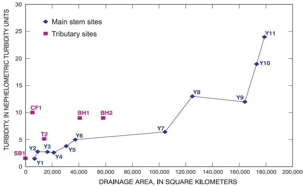
**Figure 2.** Turbidity relations with drainage area in the Yellowstone River basin and tributaries during August 2000.
